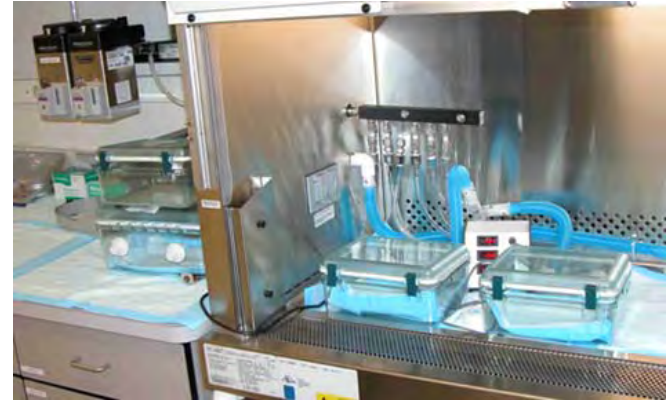
Integration with biosafety cabinet & induction boxes
